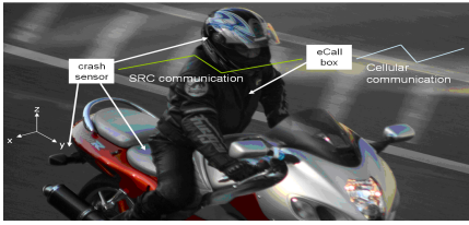
Fig. 4 Implementation of the crash sensor and eCall box on a motorbike
